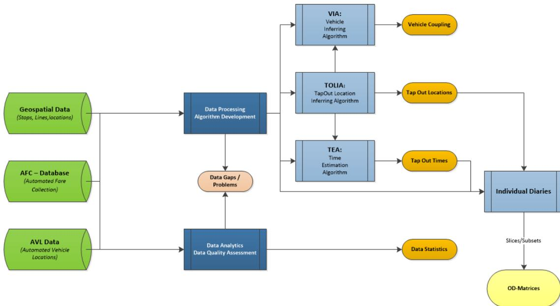
Figure 1: Schematic analysis process. Input data is represented by the three databases on the left, Processes are denoted in the middle, outputs of algorithms or processes are denoted in orange bubbles and the final output is the OD matrices formulated from Individual Travel Diaries.
