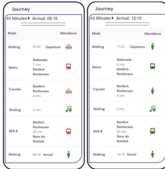
Figure 1 : User interface of the proposed predictive trip planner: The obtained journeys for two queries at rush and off-peak hours for the same couple of origin-destination. We can see in the capture at left, the train of the RER B is overloaded (pictogram in red color) at the station Denfert-Rochereau compared to the train of the midday at this station (pictogram in green color) as shown in the capture at right. We can also see the crowding level of the station when transfers are operated.
